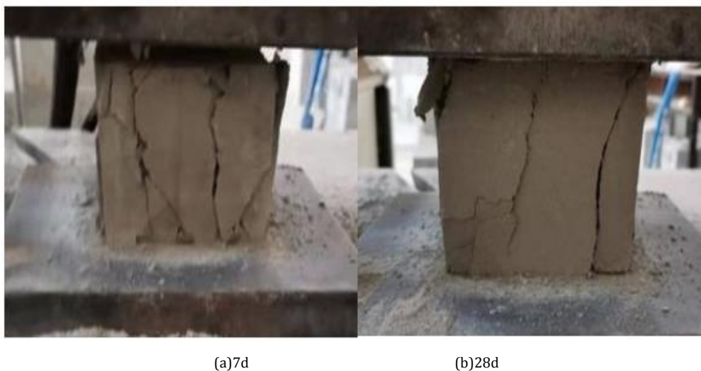
Figure 1: Failure patterns of graphite tailings foam concrete of different ages
