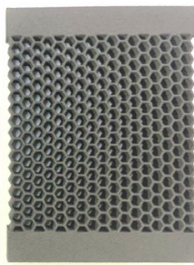
Figure 11: Hexagon honeycomb structure
