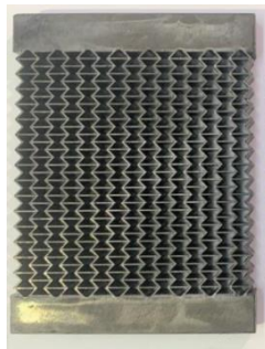
Figure 6: Specimen of re-entrant hexagonal honeycomb structure.
